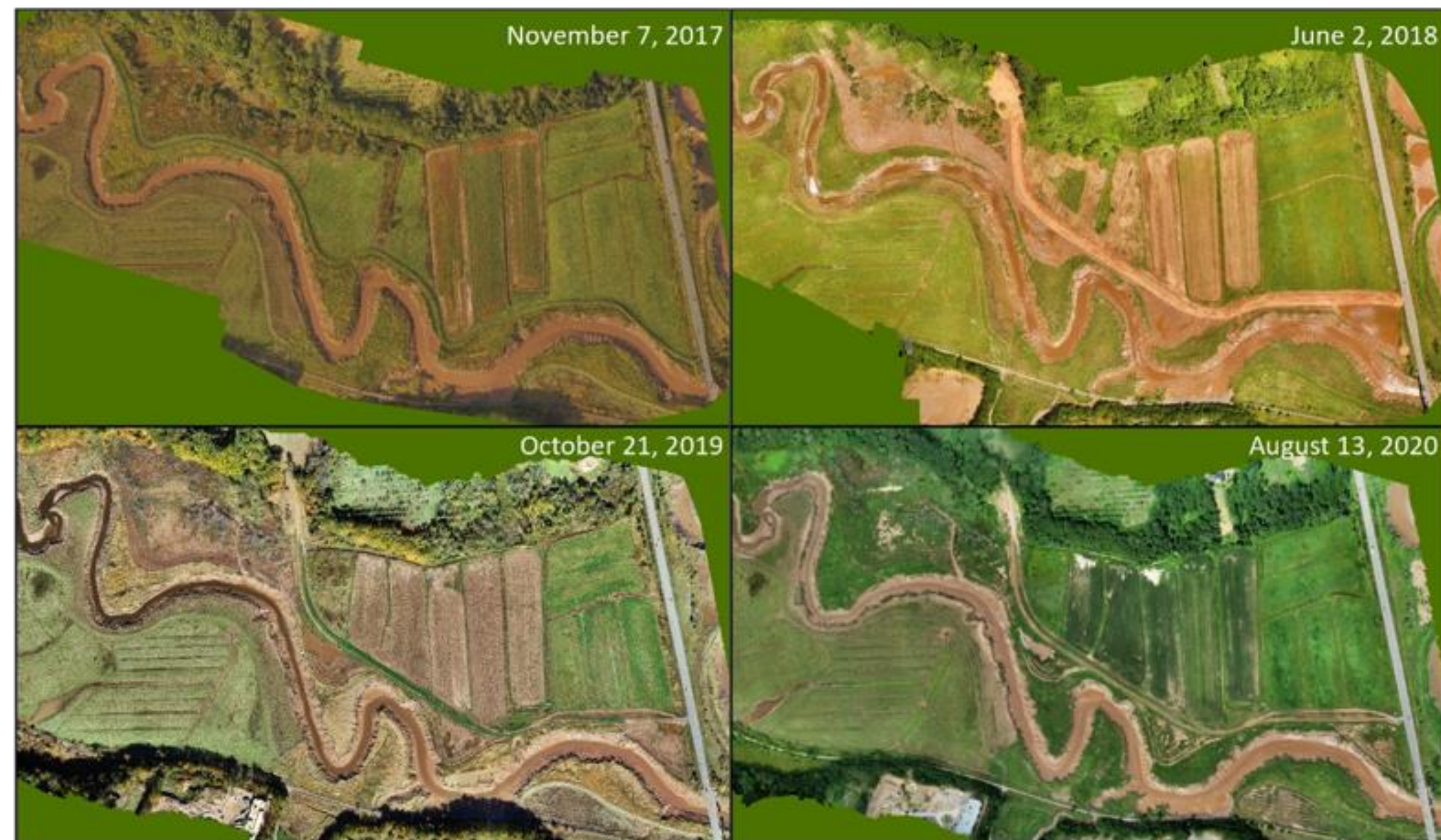
The Belcher Street managed dyke realignment site featuring a new dyke (top right) after the tides were reintroduced in May 2018, and the site two years post-breach (bottom right). The top left shows the site pre-breach and the bottom left image shows the site one-year post-breach (CBWES Inc.).
