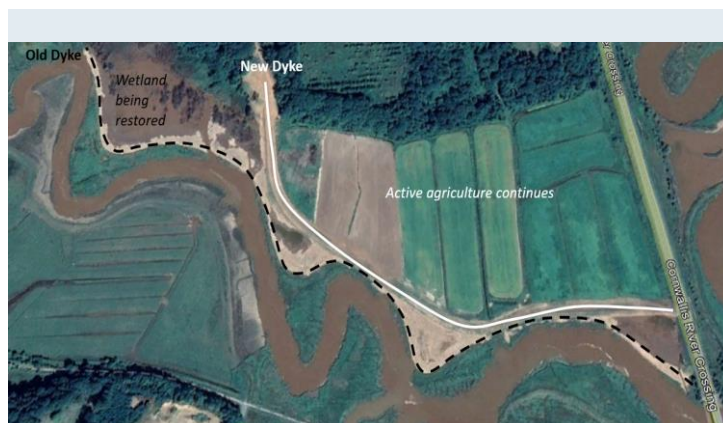
Managed dyke realignment in the Bay of Fundy. Example from realignment project on the Jijuktu'kwejk (Cornwallis) river at Belcher St. Marsh in Kentville, Nova Scotia, led by TransCoastal Adaptations.
