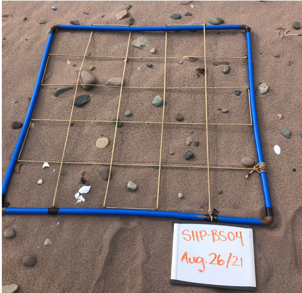
Figure 7: Example of shore substrate survey photo (step 4). Credit: CBWES Inc.
