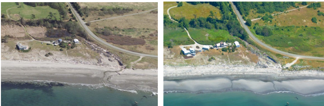
Figure 1.4.2. Groin removal on Whidbey Island WA: before and after. Although removal was not complete, erosion on the left or down-drift side is diminished due to reduced littoral drift interruption; note that the shoreline to the left of the groin is less indented or offset after removal. Credit: J. Johannessen.
