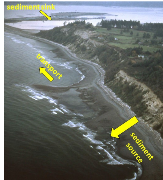
Figure K: Example of a drift cell—Goose Spit near Comox B.C. Credit: Stewardship Centre for BC.
