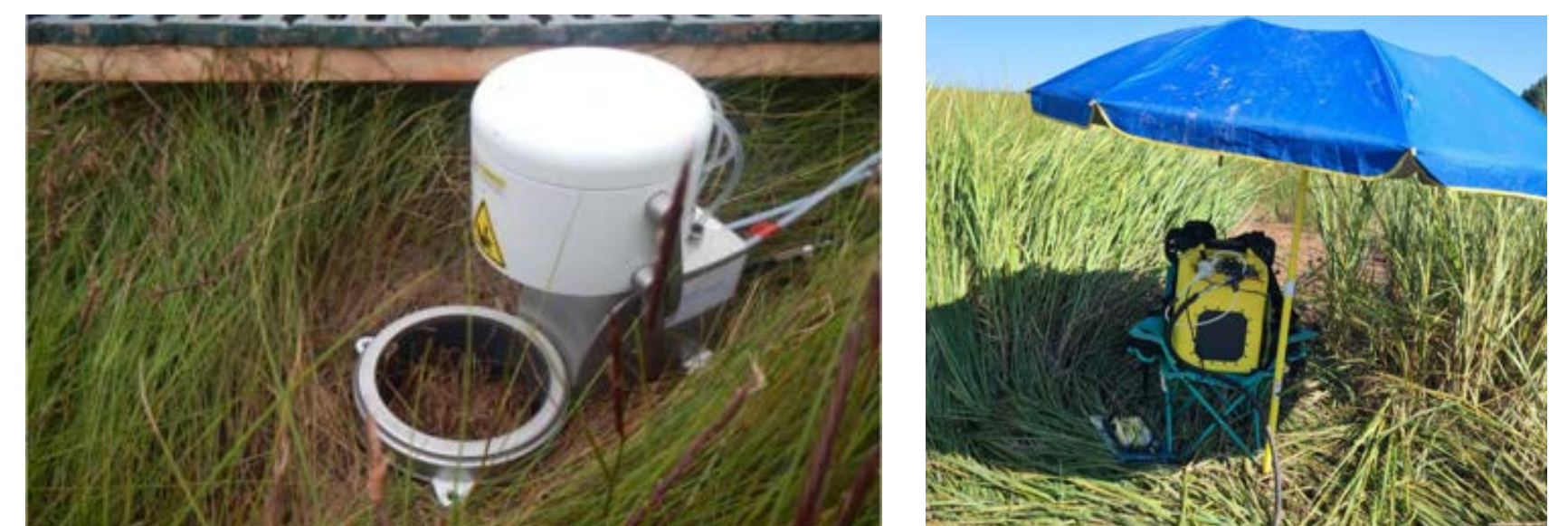
Figure 6: Eosense auto-chamber [left] (photo by Brittney Roughan); GASMET gas analyzer [right] (photo by Evan Rundle).
