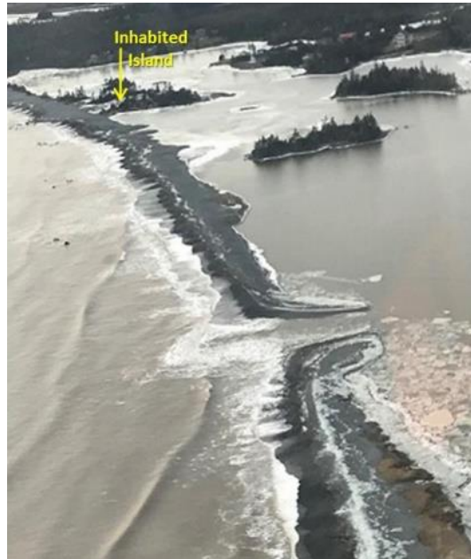
Figure 4. The breach at Big (Miseners) Lake in winter 2018. (Photo credit: NSDNR within CBCL Limited 2018)
