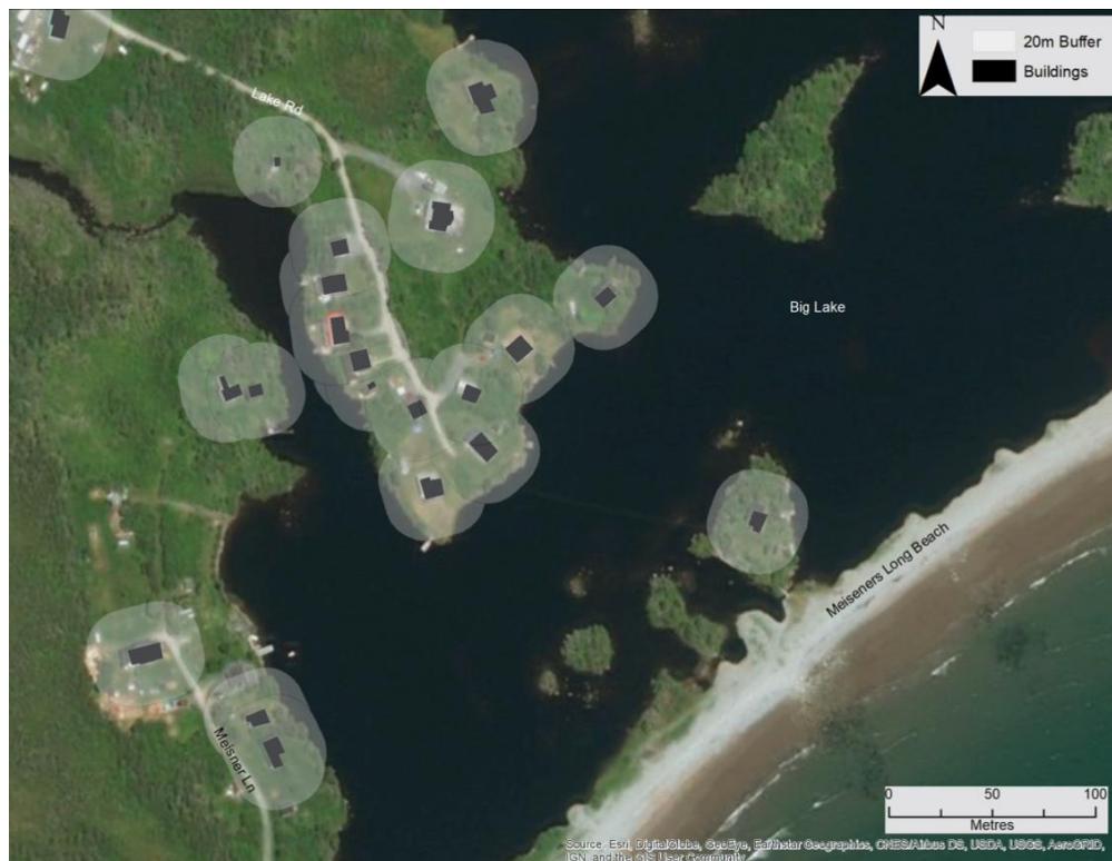
Figure 13: Infrastructure within a 20 metre shore buffer of Big Lake. All but one structure and the local road are less than 20 metres from the shore.
