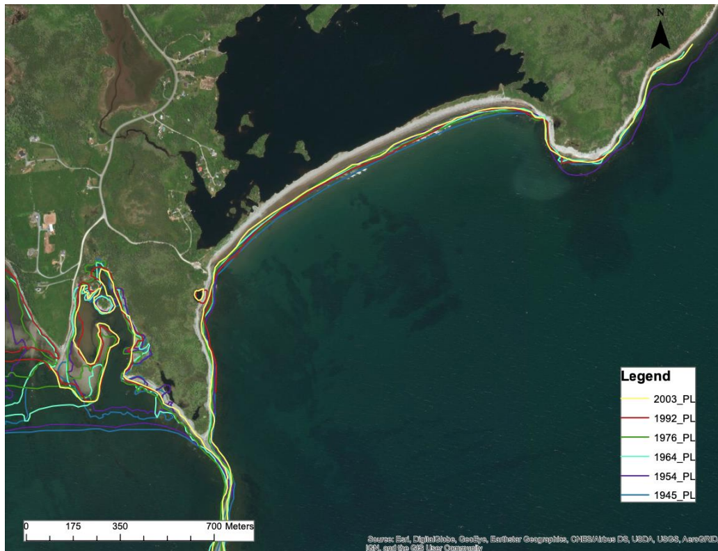
Figure 5: Historical erosion at Big Lake, NS barrier beach showing landward migration between 1945 and 2003 (Analysis and image from CBCL, 2018)
