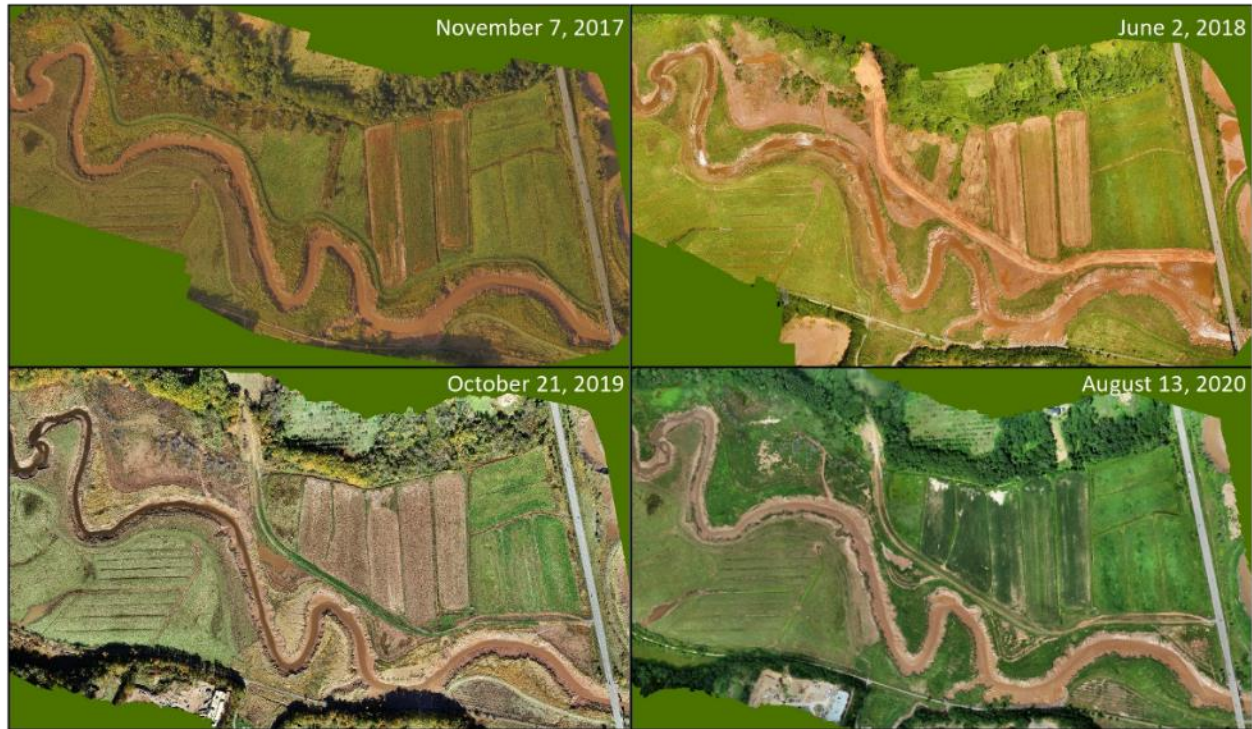
Figure 11. Belcher Street Marsh managed realignment site. Pre-restoration (top left); immediate post-construction (top right); year one post-restoration (bottom left); year two post-restoration (bottom right).
